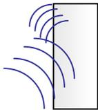
The acoustic absorption is the property which prevents sound reflection. To have a good absorption level, you need a material which is able to trap the sound waves. It is true for the porous or honeycombs materials on which the sound wave spreading is limited. The acoustical absorption is characterized by the " $\alpha$  sabine" factor. This factor is between 0 and 1. It is higher as the absorption level is increasing.
