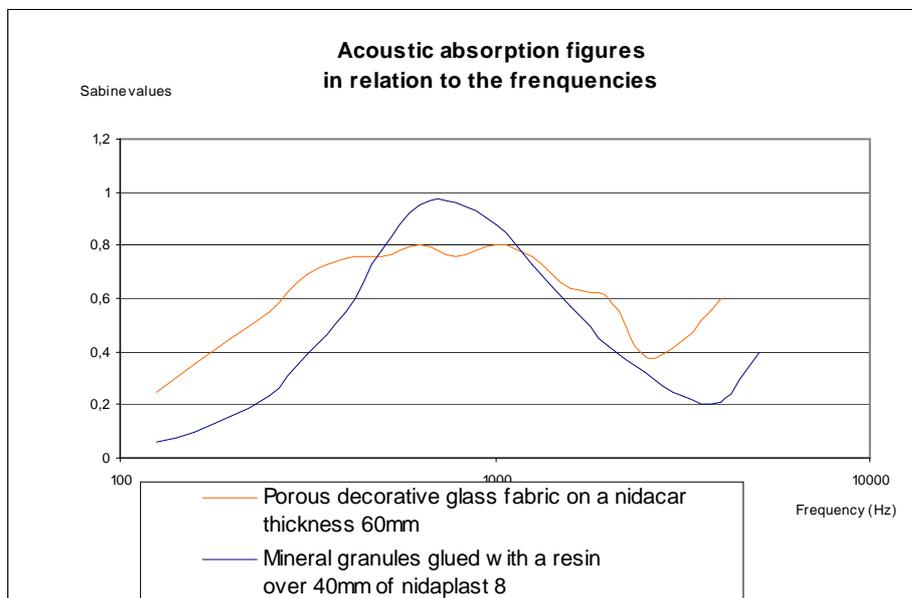
We notice a large absorption level for most of the frequencies. However, it is possible to shift the absorption level and the graph top value by playing on the **nidaplast** thickness and on the facing porosity.
