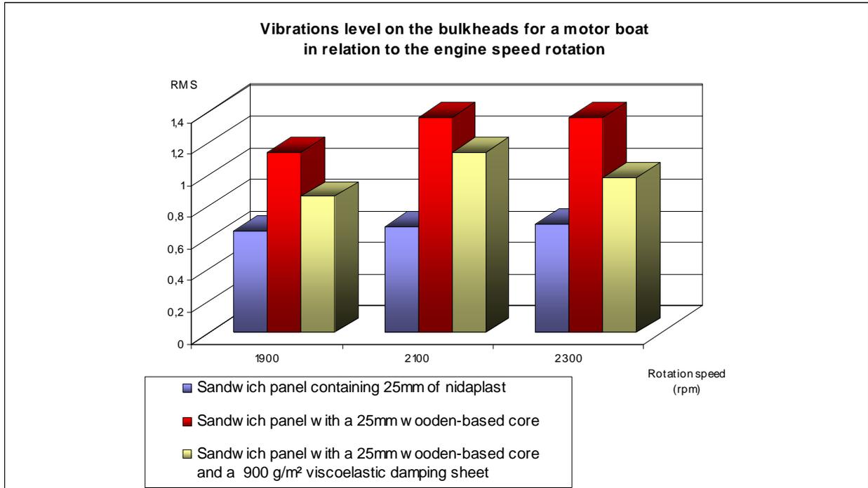
The **nidaplast** efficiency can easily be noticed on the above graphics because it is a viscoelastic product with a low modulus. Compared with a wooden core, it is possible in some case to lower by 50% the vibrations level.
